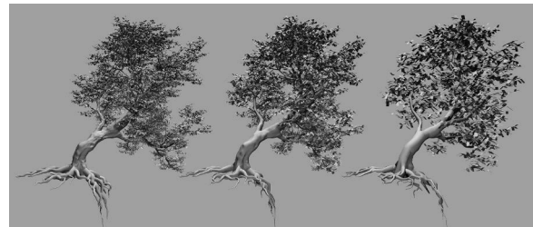
Figure 2: LOD comparison - left to right: LOD B with 657K polygons, LOD C with 49K polygons, LOD D with 7K polygons. - ©2016 Walt Disney Pictures. All rights reserved.
